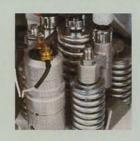
UNIT INJECTORS AND OVERHEAD Camshaft give Precision fuel Injection control. High injection pressure.
